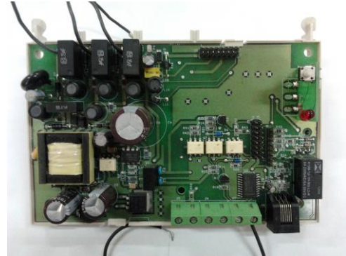
Power line communications system
